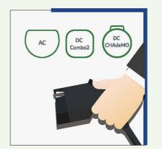
Choose the suitable cable and plug the charging cable into your vehicle and select "Start Charging" on your device screen, then press the "Start" button on the charger
