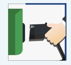
Disconnect the cable from your vehicle and return it to the charging port
